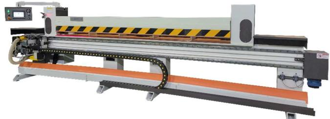
The **Veneer Sawing & Milling Machine (SawEasy 3400)** is designed for the sawing and milling of thick veneer to the desired width. After the veneer bundle is placed horizontally, its edges are sawed and milled using a stable pressure beam, a precise positioning fence and high-speed cutters, ensuring clean and squared edges for perfect splicing effects.
